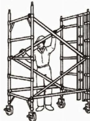
Clip diagonal braces in opposite directions as shown to from a zigzag pattern. Adjust legs to ensure tower is vertical and square and that horizontal braces are level, using a spirit level.
