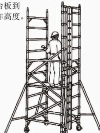
Refer the step: No.3,4,6 instruction to install upper frames with horizontal brace/diagonal brace and platform to the certain height in need.
