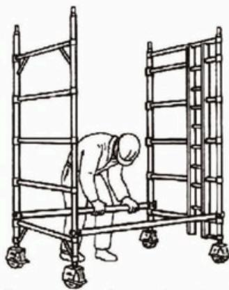
As shown in the figure, connect another cross bar to the bottom of the frame.
